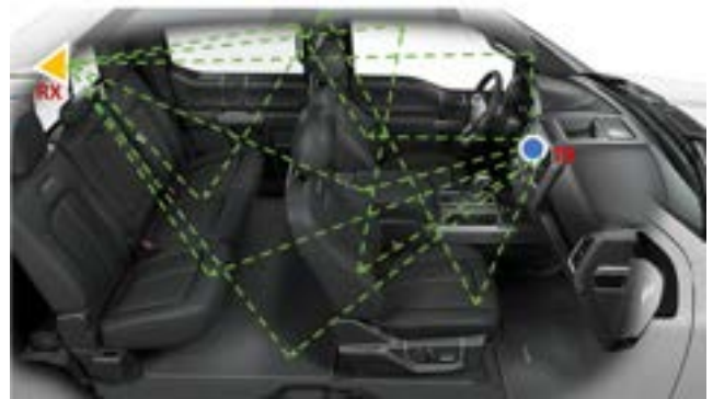
FIGURE 3. Illustration of in-car multipath propagation.
