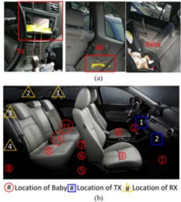
Fig. 7. Experiment scenarios. Eleven different locations of the baby, two different locations of the TX, and four different RX locations are tested. Note that baby/child in locations #1, #2, #5, #6, and #7 represent the footwell area while #8 represents the trunk area for hatchback cars. TX in #1 is fixed in the center of the dashboard while it is put inside the glove box in location #2. RX in #1, #2, and #3 are on the car liner next to the top of the car seats while location #4 denotes the cup holder on the rear door. (a) Example of the experiment setup. (b) Test scenarios in a typical car.
