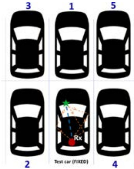
Fig. 3. Experimental setup to study the impact of external environment on the in-car CSI.
