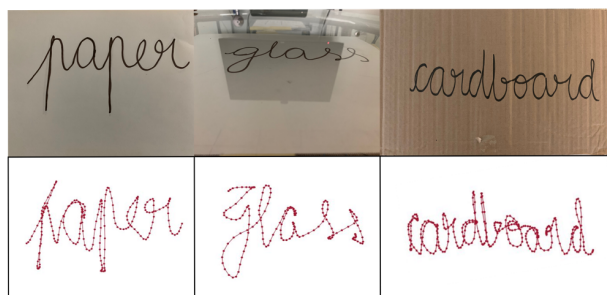
Fig. 18: Handwriting tracking on different materials
