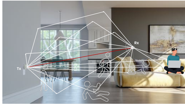
Fig. 1. An illustration of multipath propagation of Wi-Fi signals in indoor space. Human activities at different locations altering the propagation can be sensed from the received signals.
